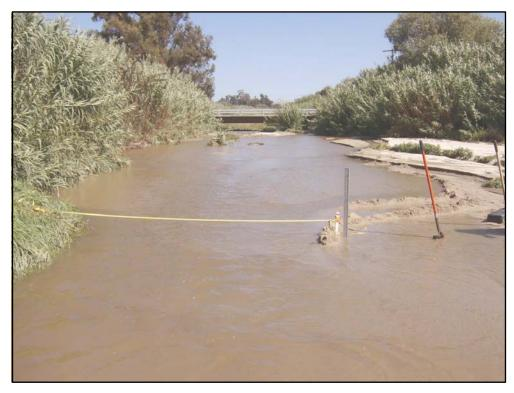
STREAM FLOW MEASUREMENTS AT SOMIS GAUGING STATION
