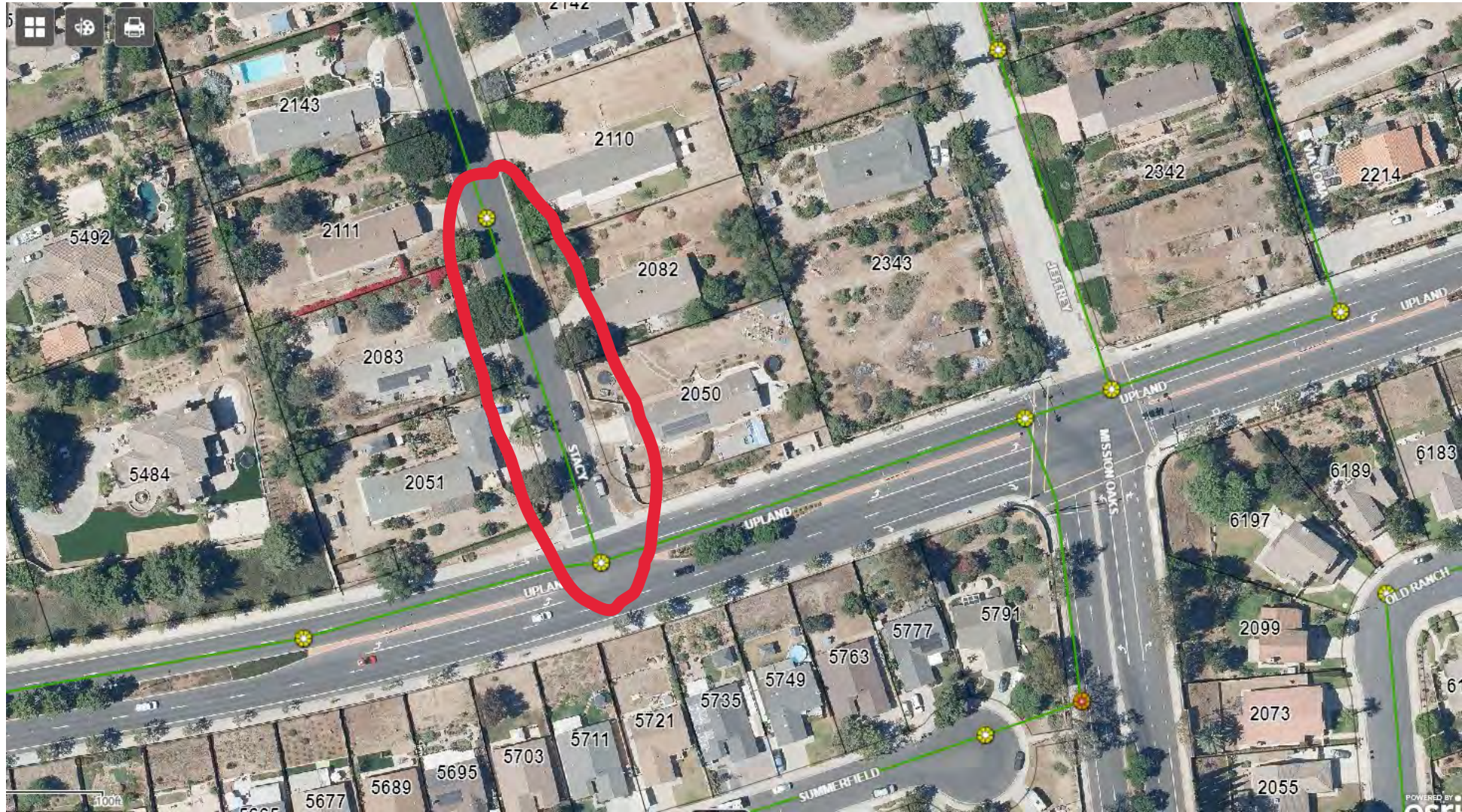
13. 2110 Stacy Lane to Upland Road. Roots intrusion in 8" sewer line between MH E46-1 and MH E46.
