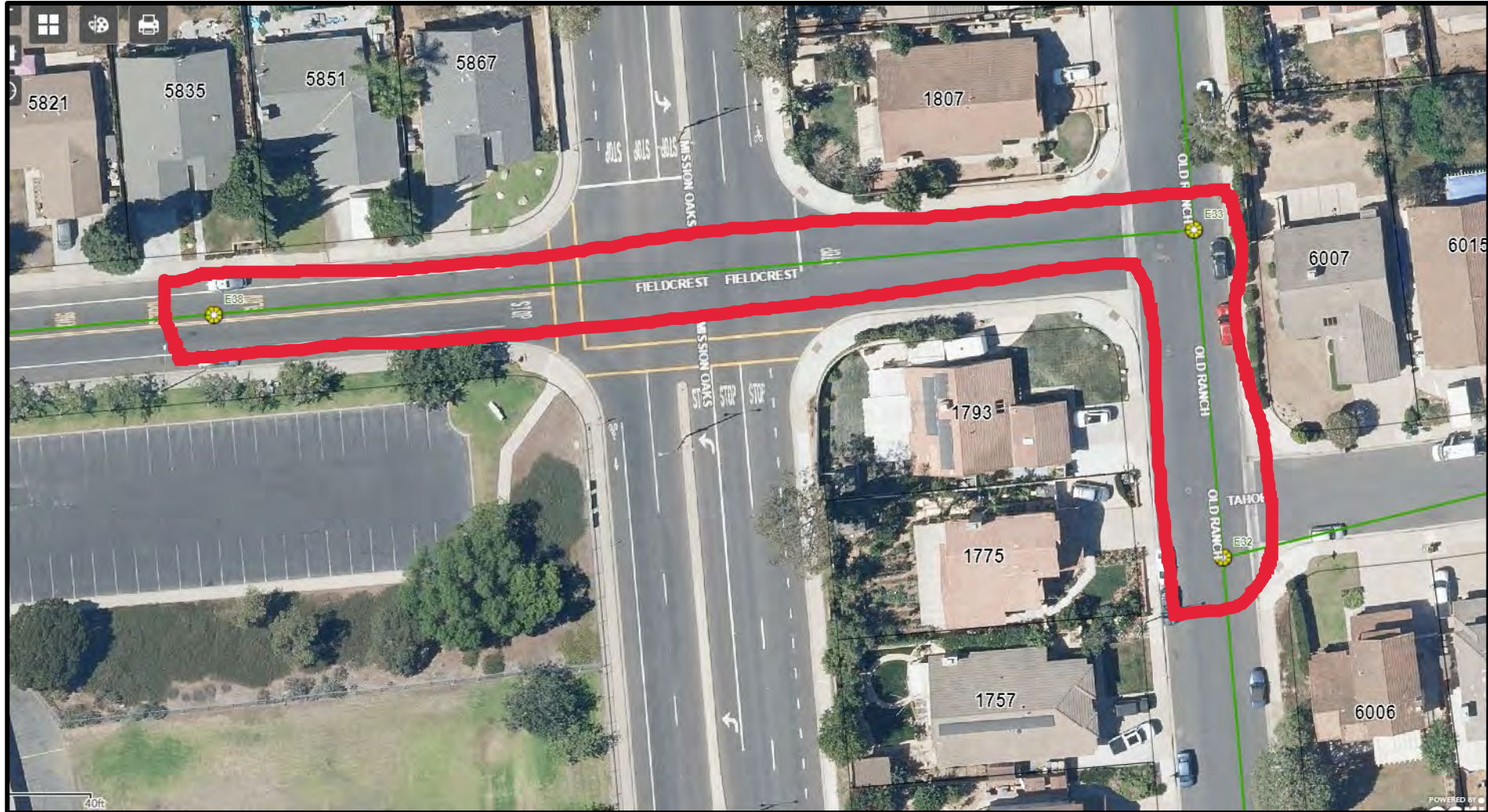
8. Fieldcrest Drive to Old Ranch Road. From MH E38 to MH E33 to E32. Heavy grease buildup and possible sag in 8" sewer line.
